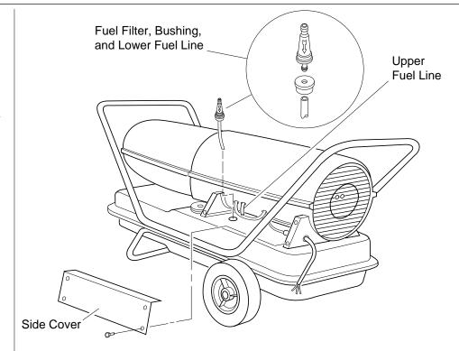
Figure 7 - Fuel Filter Removal, 100,000 BTU/Hr Model
